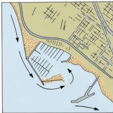
(C) After the breakwater was connected to the shore, longshore currents moved sand around the breakwater and filled the mouth of the harbor. Sand is now dredged from the harbor and pumped down the coast.
